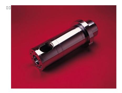
**1.** $\square$  **Reduce Cold Flakes** $\square$  ("Cold Flakes" : solidified aluminum defect pieces (scattered structure) formed in shot sleeve )
